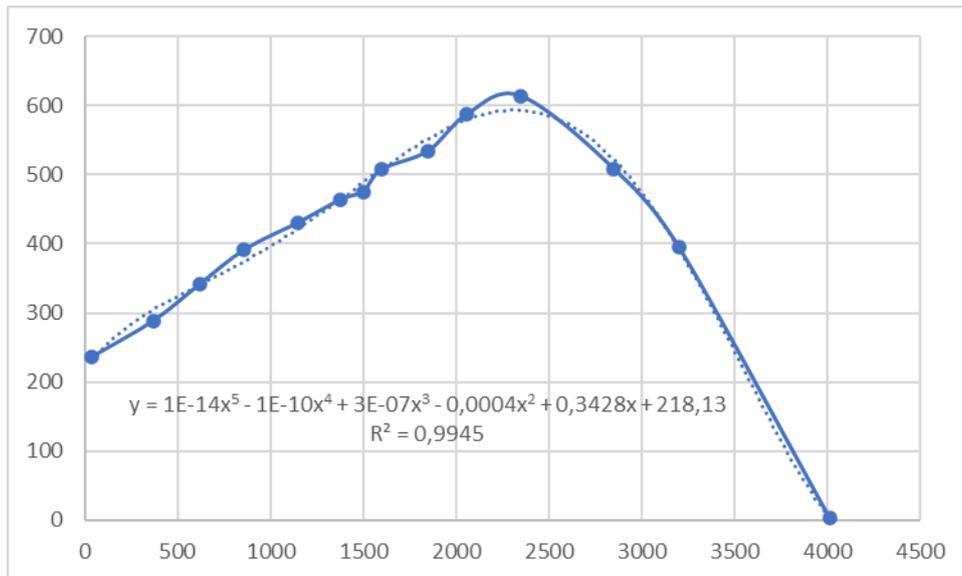
The voltage values of the joystick are first smoothed by calculating the mean value from 4 measurements. The raw values are then sent through the second-order correction function, the parameters a and b of which were determined using a spreadsheet. These values differ from module to module depending on the example and should therefore be determined by yourself. In addition, it makes sense to manually model the parameters a and b until the actual graph corresponds best to the target graph.
