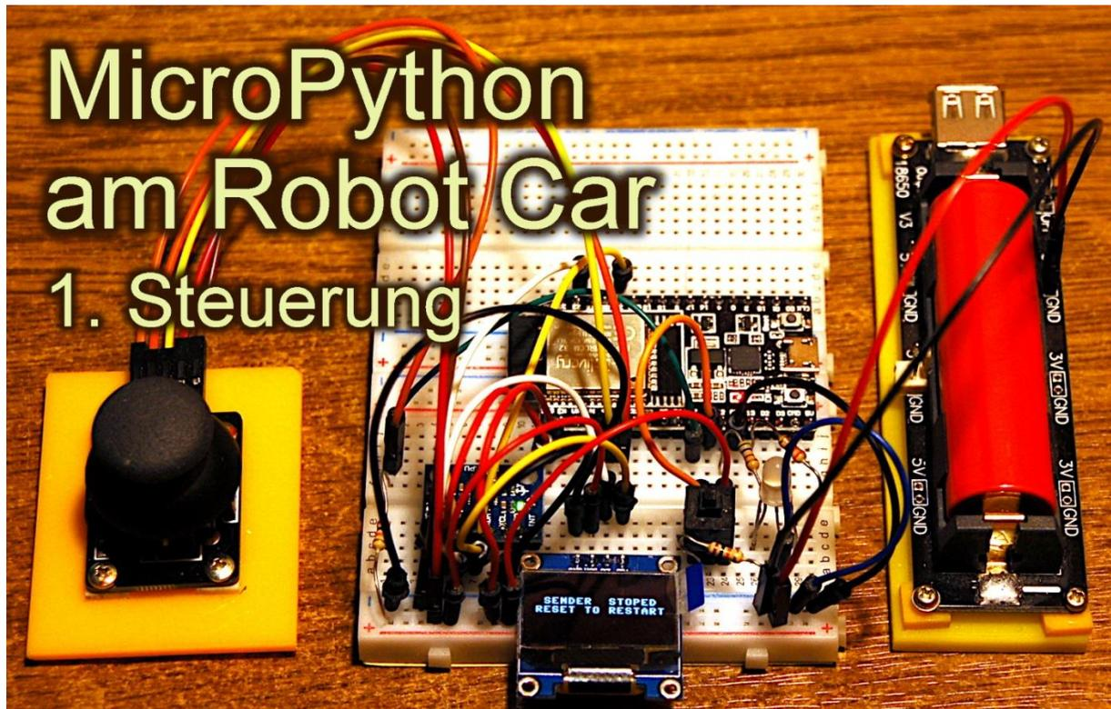
Some time ago a friend asked me if I could develop the control for a robot car in MicroPython. Sure, I said, I have to go. A WiFi-based remote control, an ESP8266 is probably sufficient and an ESP32 will be needed on the vehicle because of the numerous control lines. Build a vehicle, put a battery box on it, a motor control, for this there are special chips and a few sensors for distance measurement and path guidance, that is quite easy!
