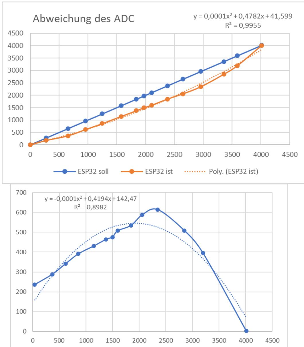
In this graphic, the difference values are plotted as a function of the raw values from the ADC. The 2nd order trend line is not optimal, but it still alleviates the measurement errors of the ADC. The following adjustment would be better, but take a look at the function term! The correlation coefficient R2 is of course almost ideal at 0.9945. Still, we stick with the quadratic function.
